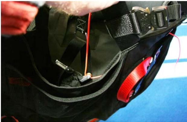
Fig. 1 – speed bar line through pulley
