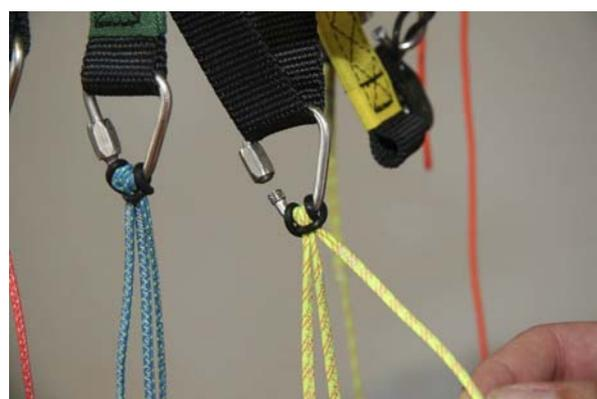
**Fig. 13: Paramotor riser with C1 quick link and both stabiliser and C1-lines**
