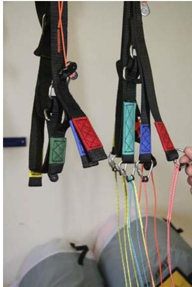
**Fig. 5: Remove the quick link**
