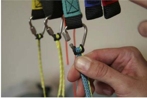
**Fig. 8: B-quick link open and showing O-ring undone**
