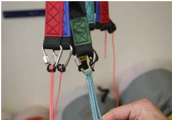
**Fig. 10: Paramotor riser with B-lines**
