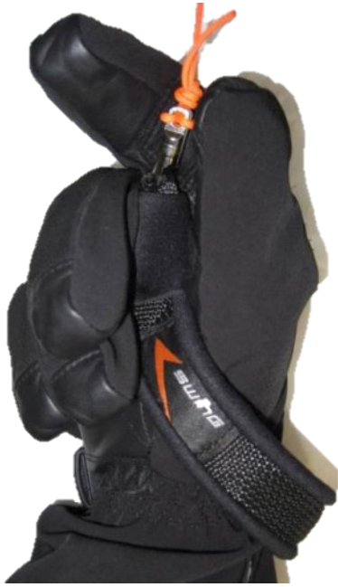
Fig. 1 Recommendation: Hand looped through the break handles
