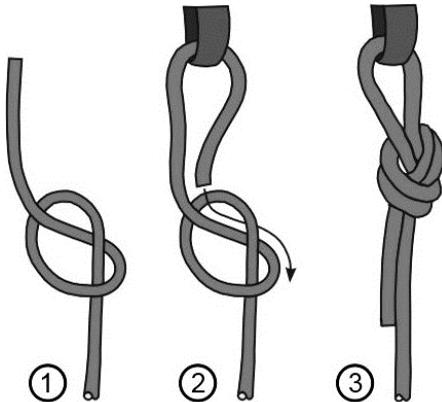
Fig. 2: Overhand knot
