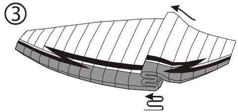
Vary slightly the final step of packing up ④, so that it is not always the middle cell which is bent. Use the neighbouring cells as well from time to time to increase the life of the fabric, particularly in the middle part.
