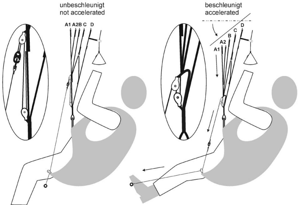
**Fig. 5:** How the Arcus 7 speed system works
