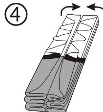
When you are completing the final part of packing, we recommend that you put the internal protection bag under the glider to minimise abrasion on the ground.
